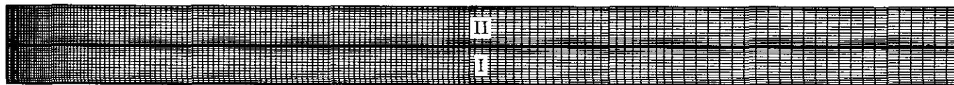
FIG. 5. Computational grid for the flow over a backward-facing step in a two-dimensional channel for Re = 700 . Each subdomain contains 21 \times 172 grid points; the buffer domain is not included.
